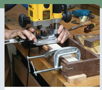
**CLAMP A SHORT BOARD** to the box wall to support the base of the router. Use an edge guide to rout the long rear wall of the mortise.
